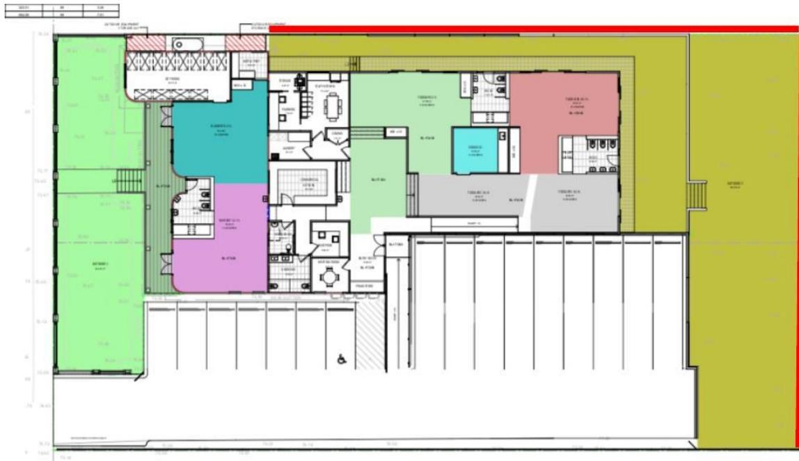
As shown in red in the above diagram a 2.1m solid continuous barrier is recommended to be constructed to the boundary of the proposed rear external play area to mitigate noise (SEE, p. 55).
